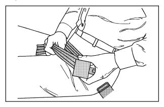
When you sit in a center front seating position, you have a lap safety belt, which has no retractor. To make the belt longer, tilt the latch plate and pull it along the belt.
